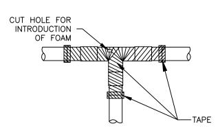
IF REQUIRED, SLIDE PVC EXTENDERS OVER END OF PIPE PRIOR TO TEE BEING WELDED INTO POSITION.
