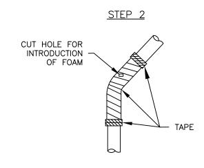
TEST ALL JOINTS AS REQUIRED. POSITION AND SECURE PVC ELBOW COVER. CUT SMALL OPENING IN COVER FOR INTRODUCTION OF FOAM.
