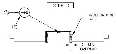
APPLY UNDERGROUND TAPE WHERE PVC SLEEVE AND CASING MEET. PROVIDE FOR A MINIMUM OVERLAP OF 2". REFER TO CHART BELOW FOR FOAM AMOUNT BASED ON JACKET SIZE. POUR FOAM INTO OPENING. WHEN FOAM REACTS, TEMPORARILY SEAL THE OPENING WITH DUCT TAPE TO MAXIMIZE INSULATION IN CAVITY.
