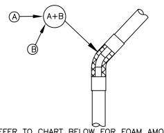
REFER TO CHART BELOW FOR FOAM AMOUNT BASED ON JACKET SIZE. POUR FOAM INTO OPENING.
