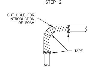
TEST ALL JOINTS AS REQUIRED. POSITION AND SECURE PVC ELBOW COVER. CUT SMALL OPENING IN COVER FOR INTRODUCTION OF FOAM.
