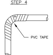
TRIM OFF EXCESS MATERIAL AFTER CURING IS COMPLETE. WRAP FITTING WITH PVC TAPE AS SHOWN.
