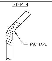
TRIM OFF EXCESS MATERIAL AFTER CURING IS COMPLETE. WRAP FITTING WITH PVC TAPE AS SHOWN.
