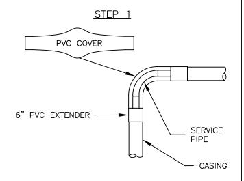
IF REQUIRED, SLIDE PVC EXTENDERS OVER END OF PIPE PRIOR TO ELBOW BEING WELDED INTO POSITION.
