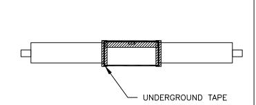
TRIM OFF EXCESS MATERIAL AFTER CURING IS COMPLETE. APPLY ADDITIONAL UNDERGROUND TAPE TO HOLE IN PVC SLEEVE.
