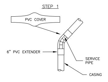
IF REQUIRED, SLIDE PVC EXTENDERS OVER END OF PIPE PRIOR TO ELBOW BEING WELDED INTO POSITION.
