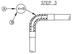
REFER TO CHART BELOW FOR FOAM AMOUNT BASED ON JACKET SIZE. POUR FOAM INTO OPENING.
