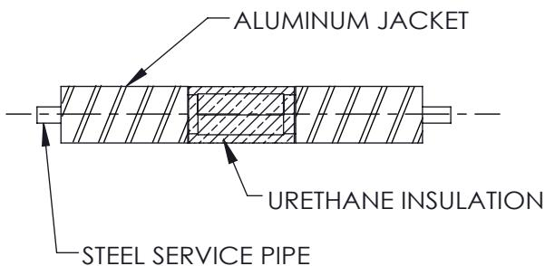
APPLY URETHANE FOAM INSULATION IN PLACE AND SECURE.
