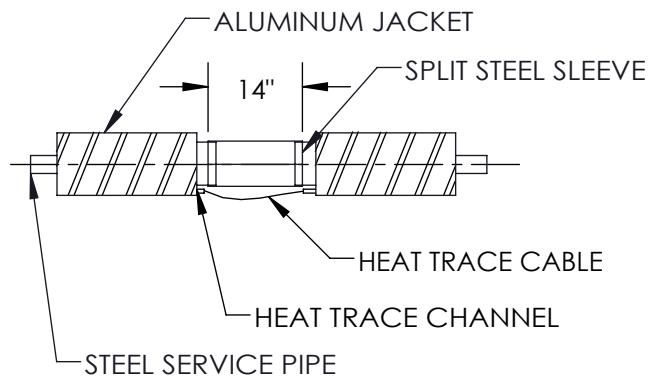
FIT 10 GA. SPLIT STEEL SLEEVE ONTO CONDUIT AND WELD IN PLACE WITH TWO CIRCUMFERENTIAL AND ONE HORIZONTAL WELD. AIR TEST TO 15 PSI. FEED HEAT TRACE CABLE THROUGH CHANNEL TO ADJOINING PIPE SECTION.
